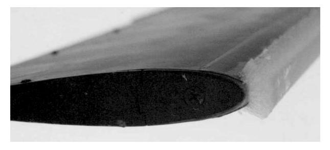
Rime ice which has formed on the leading edge of a helicopter rotor blade. Note that the ice builds up on the leading edge of the blade leaving the top and bottom surfaces virtually ice free. The ice build-up acts as a spoiler, disrupting the airflow over the aerofoil surface and drastically affecting the lift produced.
