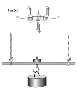
If the weight is increased the bending loads imposed on the plank will increase until the plank breaks under the increased load [Fig 5.2 top].
