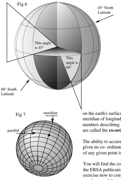
The parallels are numbered north and south of the equator according to the angle formed between the plane of the equator and a line from any point on that parallel to the centre of the earth [Fig 6].
