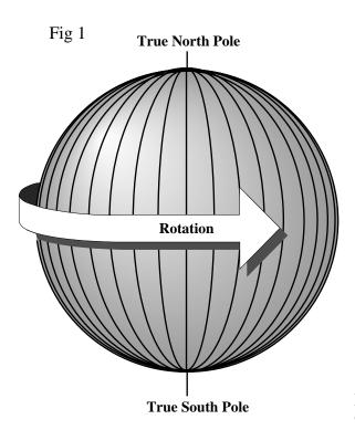
The true north and true south poles and the equator form the basis for the grid of latitude and longitude. This grid is used for defining position on the surface of the earth.
